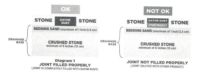
DO NOT USE WHEN STONES ARE INSTALLED OVER A CONCRETE SLAB. DO NOT USE FOR VEHICULAR TRAFFIC.
